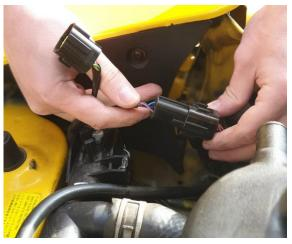
If you have removed the motor connectors from the body clip, it can now be clipped back in. The two sets of plugs/sockets can be cable tied together to keep them secure.
